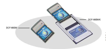
DCF-660W ComplactFlash Type I card (left)and DCF-660WK kit with PCMCIA converter that plugs this CompactFlash card to a network PC (right)
