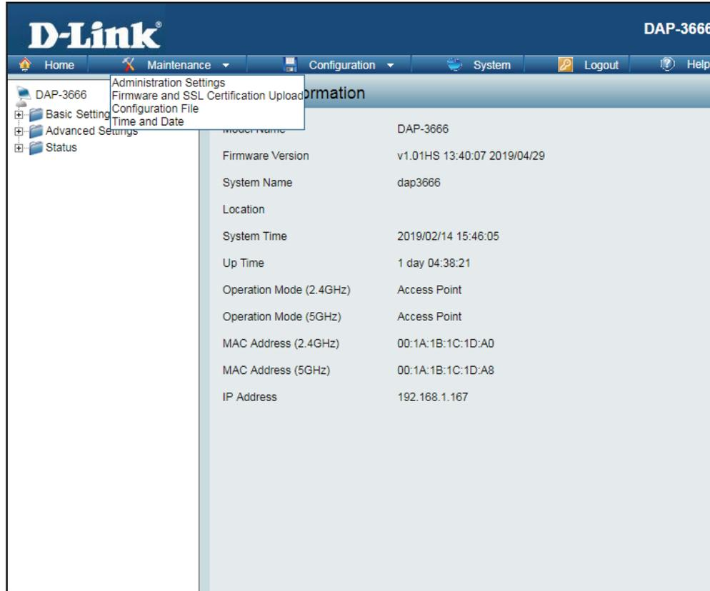
The screenshot displays the D-Link DAP-3666 Web User Interface. The top navigation bar includes Home, Maintenance, Configuration, System, Logout, and Help. The Maintenance section is expanded, showing a list of settings:
