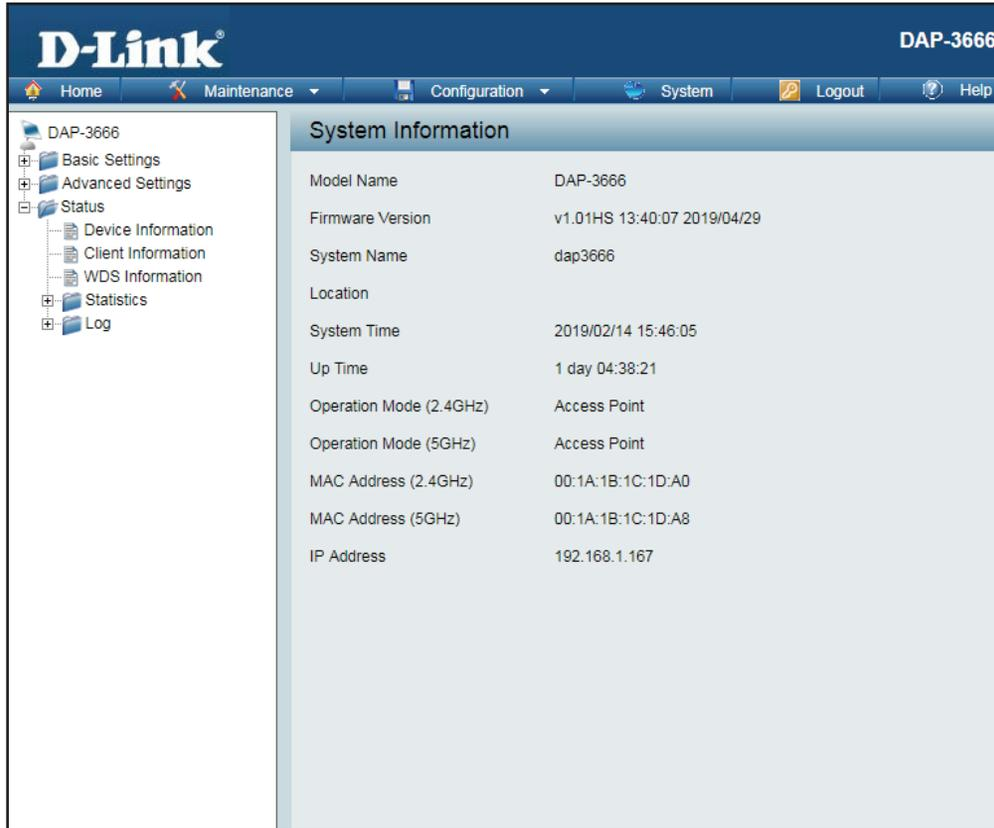
The screenshot displays the D-Link DAP-3666 Web User Interface. The top navigation bar includes Home, Maintenance, Configuration, System, Logout, and Help. The left sidebar shows a tree view with DAP-3666 expanded, containing Basic Settings, Advanced Settings, Status, Device Information, Client Information, WDS Information, Statistics, and Log. The main content area is titled "System Information" and displays the following details:
