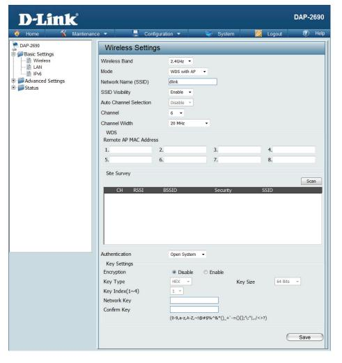
Remote AP MAC Allows selection of the channel width you would like to operate in. **20 MHz** and **Auto 20/40 MHz** allow both 802.11n and non-802.11n **Address:** wireless devices on your network when the wireless mode is Mixed 802.11 b/g/n in 2.4G and Mixed 802.11 a/n in 5G. 802.11n wireless devices are allowed to transmit data using 40 MHz when the channel width is **Auto 20/40 MHz**.
