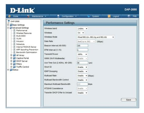
Beacon Interval Beacons are packets sent by an access point to synchronize a wireless network. Specify a value in milliseconds. The default (100) is (40-500): recommended. Setting a higher beacon interval can help to save the power of wireless clients, while setting a lower one can help a wireless client connect to an access point faster.
