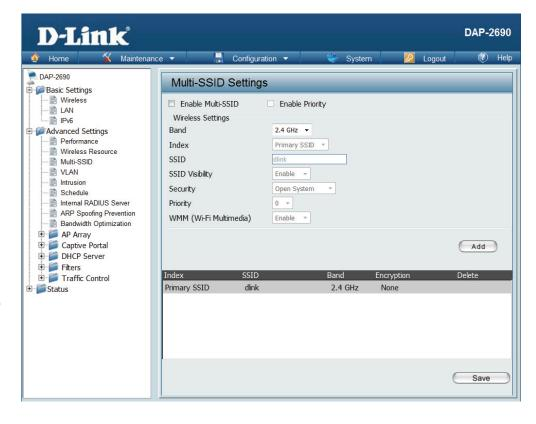
**Priority:** When the Enable Priority check box is checked at the top of this window, this drop-down menu is used to select a priority between **0** and **7**.
