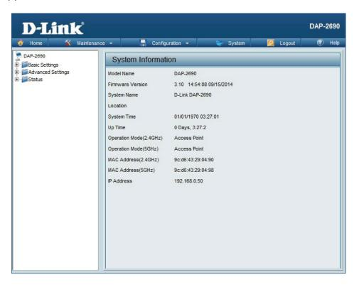
Alternatively, click the **Save and Activate** option on the Configuration drop-down menu at the top of each DAP-2690 window. This will cause the DAP-2690 to save and reboot.
