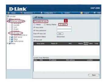
**Step 2:** Click <u>Scan</u> button to search the existing array, and enter the array password to join it.
