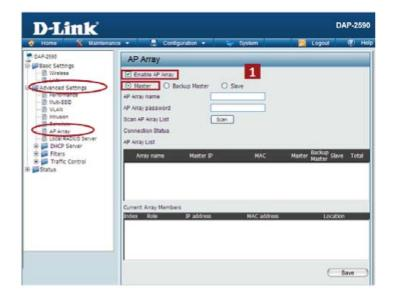
Step 2: Set up the AP Array name and password.
