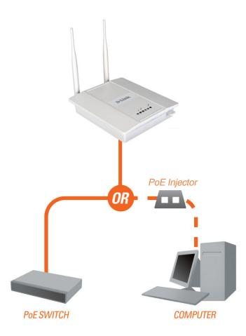
Connect one end of an Ethernet cable (included with your access point) to the LAN port on the DAP-2360 and the other end of the Ethernet cable to either your computer or to your PoE switch. The AP can be powered on by a PoE switch or by the DPE-101GI.
