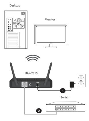
1. Connect the power adapter to the receptor on the rear panel of the DAP-2310 and then plug the other end of the power adapter to a wall outlet or power strip. The power LED will turn ON to indicate proper operation.
