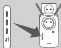
If the Smart Signal LED has a single amber bar after the connection process has finished, the DAP-1635 has established a poor quality connection. To improve the connection quality, the DAP-1635 should be relocated to a wall outlet closer to the source wireless router or AP. The more lit bars on the Signal LED, the better the wireless signal.
