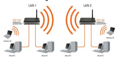
Connecting two separate LANs together through two DAP-1160 units (Wireless PCs can access the DAP-1160 units)
