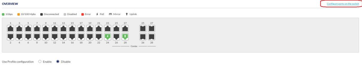
Here you also can see if a port is connected, the connection speed and when supported if PoE is delivered.
