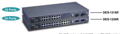
DES-1218R switch (top) with 16 10/100Mbps ports. DES-1226R switch (bottom) with 24 10/100Mbps ports. Optional modules providing 2 Gigabit fiber ports are shown inserted in the open slots on the right-hand side.
